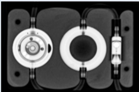
X-ray image of Valve Board with *proGAV 2.0* with prechamber, lumbar right (pressure rating of *proGAV 2.0* - 20 cmH<sub>2</sub>O pressure rating of *SHUNTASSISTANT 2.0* - 25 cmH<sub>2</sub>O)
