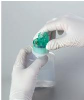
Place Ecoflac® Mix on the upright standing container and puncture the port. No need to rotate the spike.
