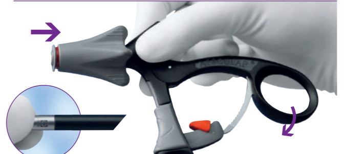
IV Connect shaft and handle Hold the shaft firmly by its tip and the handle behind the rotation knob. Push the shaft into the handle until it locks in place and the red ring disappears. Important: Do not hold on to the movable handle component.
